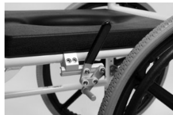
Pic. 4: Mounting of brakes to the frame
